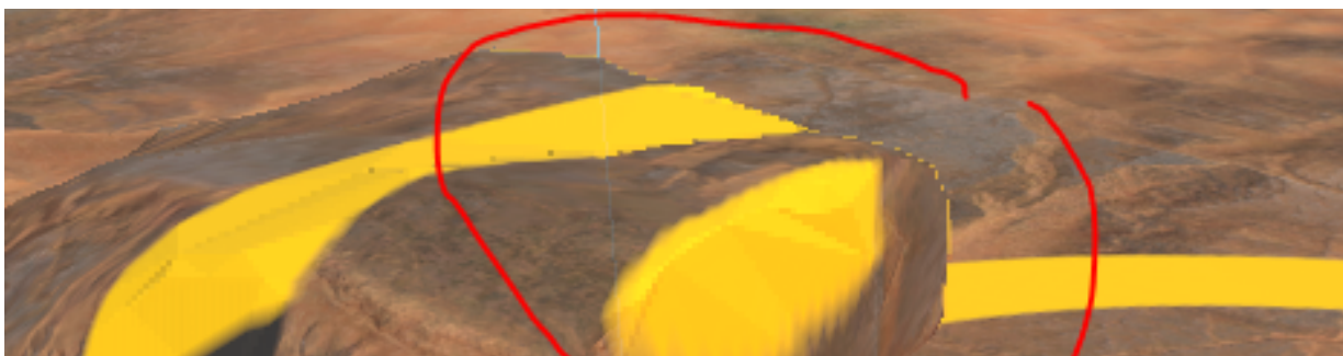
HQ Sampling disabled: 2x2px artifacts around edges in the depth buffer.
